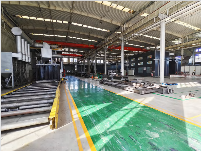
Include Sand and Ball Blasting Machine, Painting and Powder Coating Production Line (Control Ambient Air for High quality)
