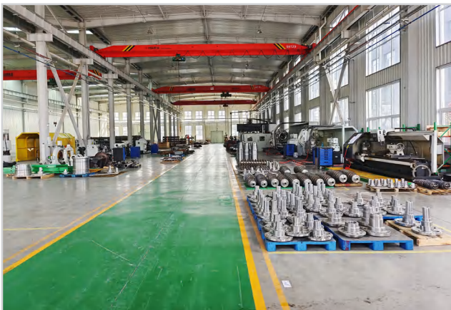
Centrifuge and Pumps Production by CNC lathe, CNC machining center and Balance Machine etc.
